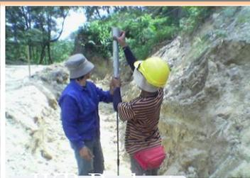
JKR Probe to confirm bearing capacity of soil
