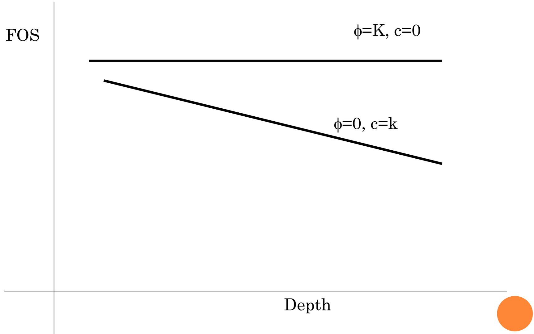
Civil engineers are expected to make calculations to check the safety of slopes (slope stability analysis), it involves determining and comparing the shear stress developed along the most likely rupture surface with the shear strength of the soil. Generally, the factor of safety is:
