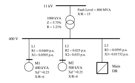
A distribution system has components and parameters as seen below. Find the fault current if fault occurs at
