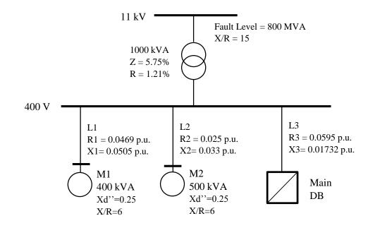
Using the separate R and X diagram, determine the fault current for fault at
