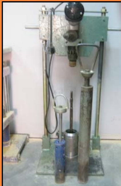
SOIL COMPACTION TEST
