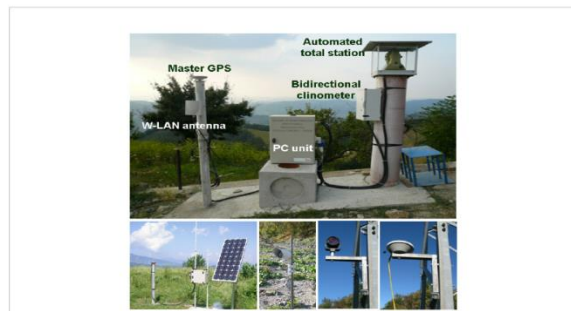
Fig. 2. Integrated monitoring system for unstable slopes: master unit at the top; below a GNSS remote site for continuous monitoring, reflectors and reference prism/GNSS
