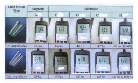
Diagram 5.2: Illuminance Test with Parabolic Reflector
