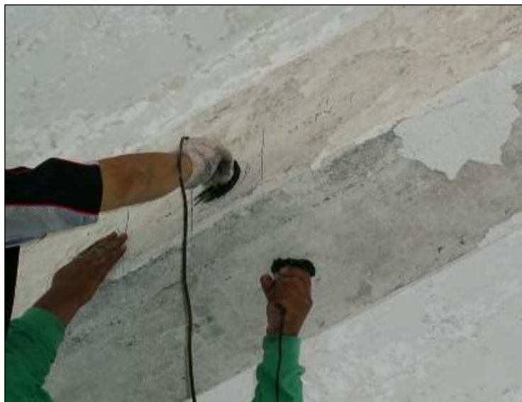
Figure 5.4: Arrangement of transducers for semi-direct transmission.
