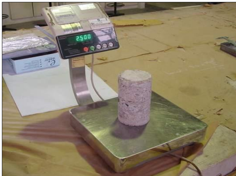
Figure 10.7: Weighing the specimen on a scale.
