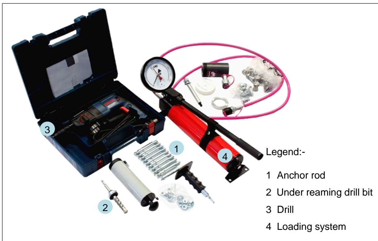
Figure 15.2.2: Pull-out testing equipment for inserts on hardened concrete.
