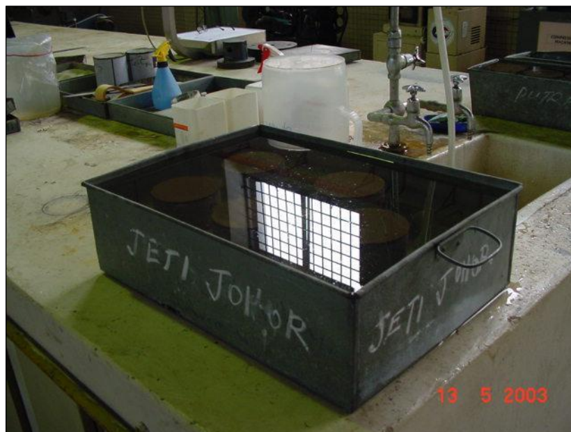
Figure 3.7: Store the specimen in water.
