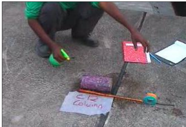
Figure 6.3: Spraying phenolphthalein solution on a core sample.
