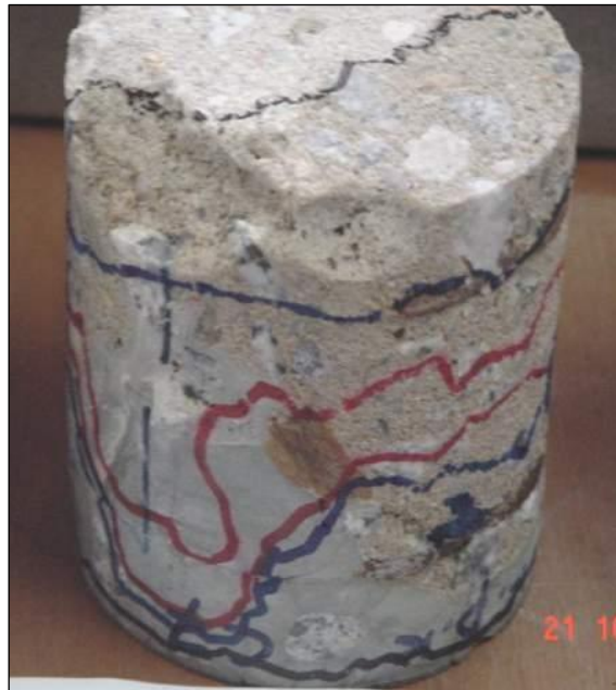
Figure 11.7: Draw water rising profile on specimen surface.
