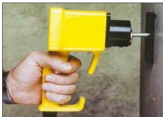
Figure 15.5.4: Measuring the exposed probe length.
