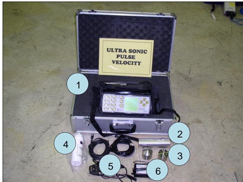
Figure 5.1: UPV test components.
