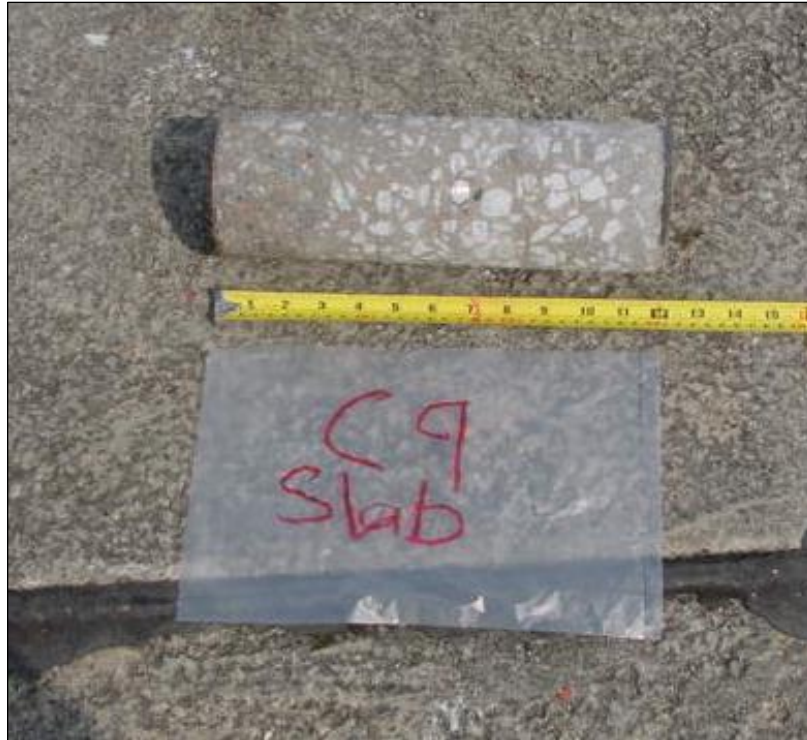
Figure 6.2: Core sample ready for carbonation test.
