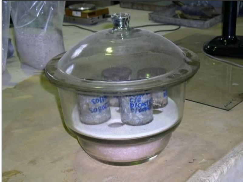
Figure 10.6: Storing specimens in a desiccator.
