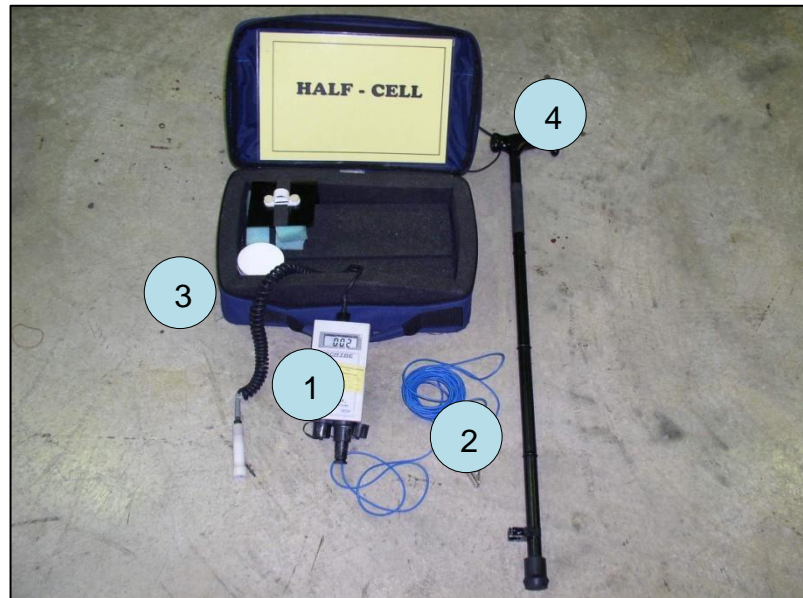
Figure 7.1: Half-cell potential test equipment.
