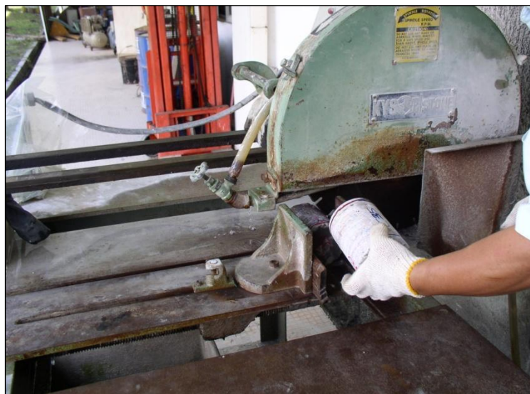
Figure 3.5: Grinding of specimen using grinding machine.
