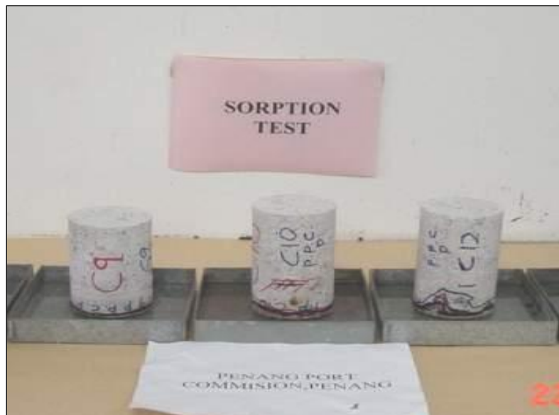
Figure 11.6: Placing specimens on the tray with water at 1-2mm height.
