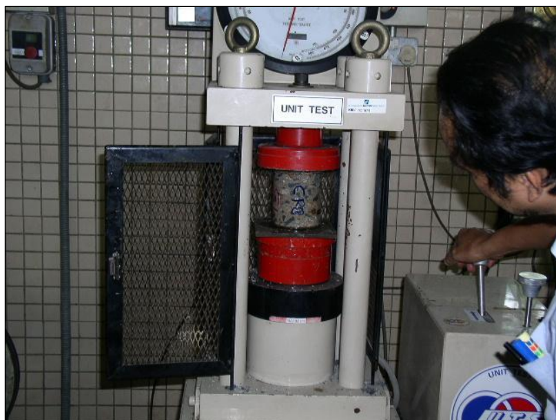
Figure 3.8: Testing for core compressive strength.
