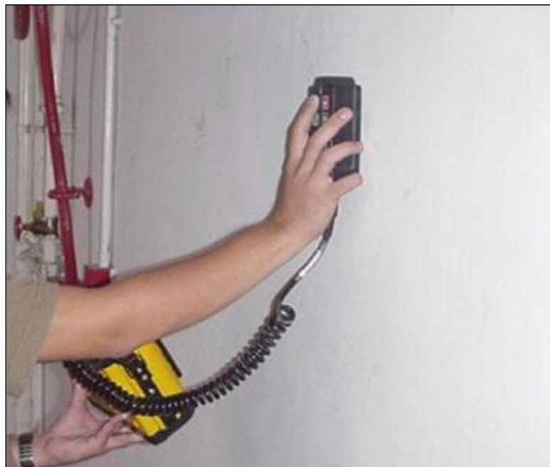
Figure 2.3: The position of head to scan over the concrete surface.
