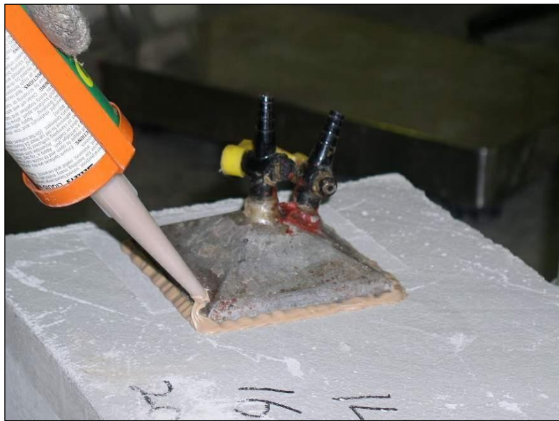
Figure 8.2: Fixing the cap onto concrete surface.
