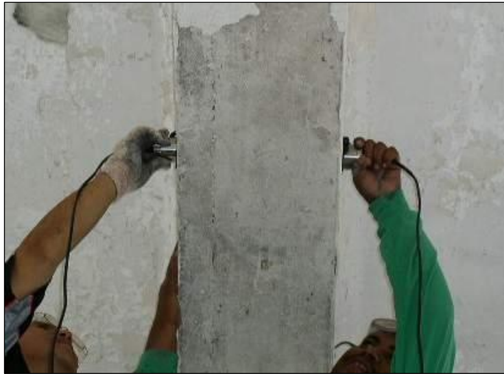
Figure 5.3: Arrangement of transducers for direct transmission.
