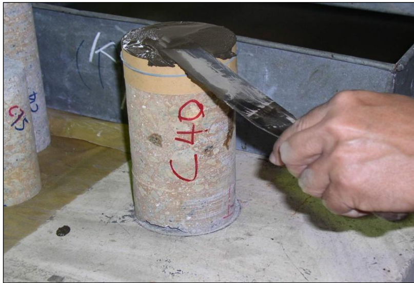
Figure 3.6: Capping the ends of specimen.
