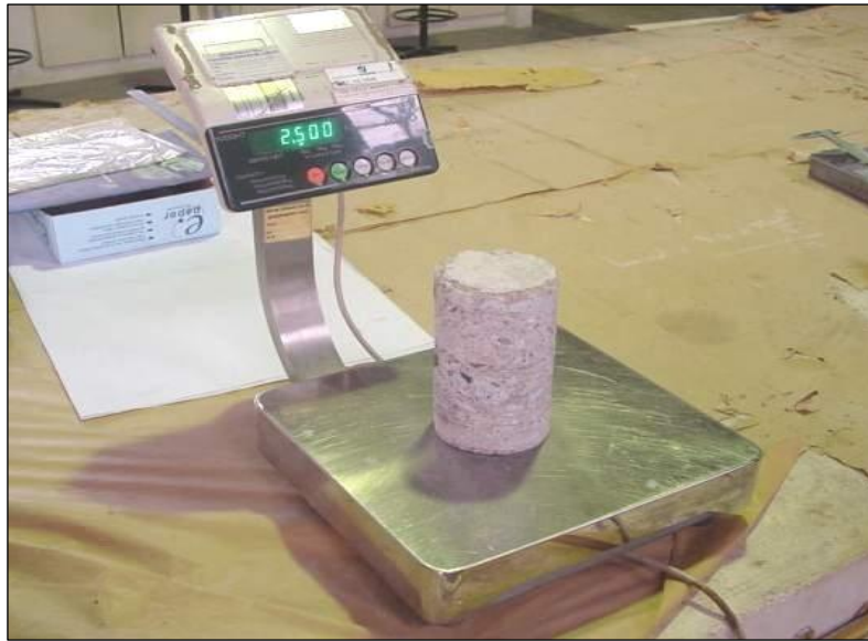
Figure 11.5: Weigh the specimen on a balance.
