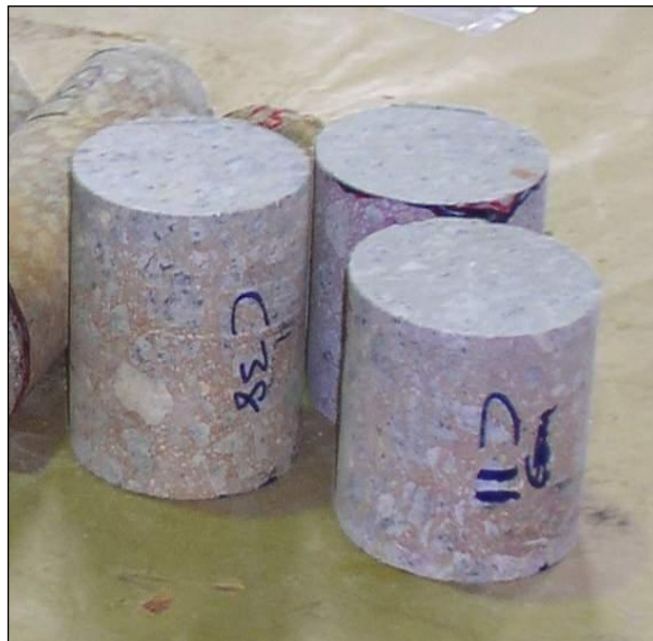
Figure 10.5: Cylinder specimens ready for water absorption test.
