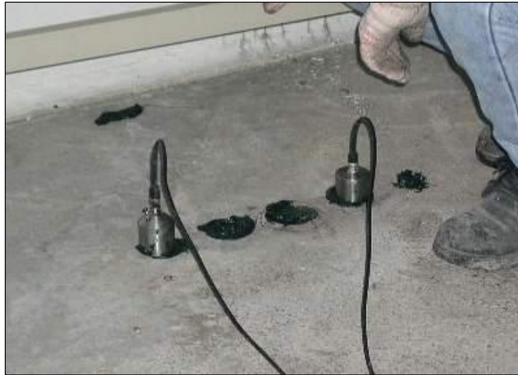
Figure 5.5: Arrangement of transducers for indirect transmission.
