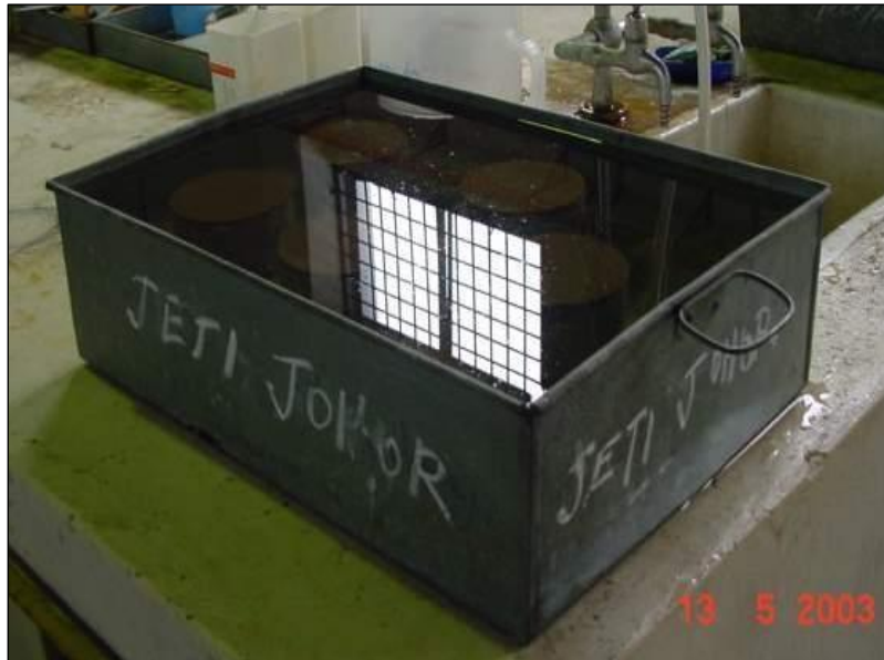
Figure 10.8: Submersion of specimen in water.
