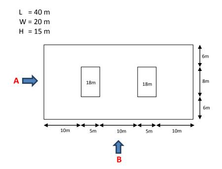
Design a lightning protection system for this building using the protective angle method with 500 mm air terminals. Choose the Class IV lightning protection level (LPL).
