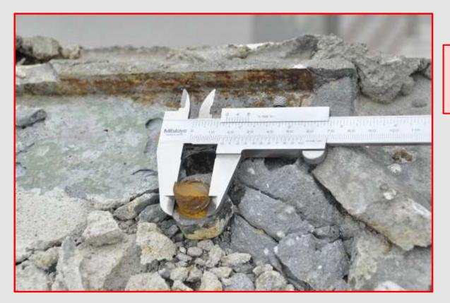
20mm diameter Type 1 Deformed Bars were used as anchorage
