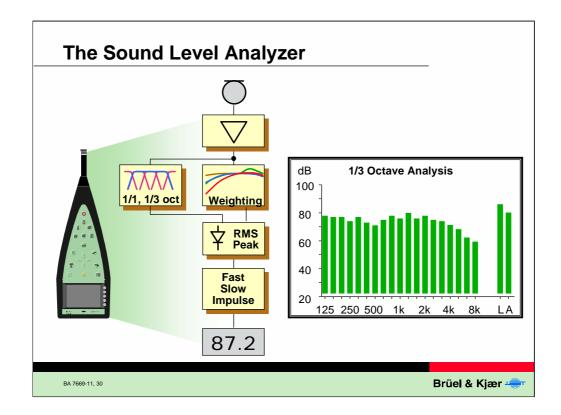
The most advanced sound level meters act more like an ordinary sound analyzer having both a parallel filter bank and a selection of weighting filters.
