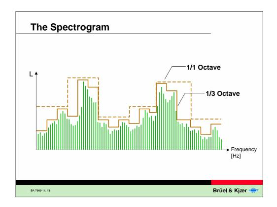
A detailed signal with many frequency components show up with a filter shape as the dotted curve when subjected to an octave analysis. The solid curve shows the increased resolution with more details when a 1/3 octave analysis is used.
