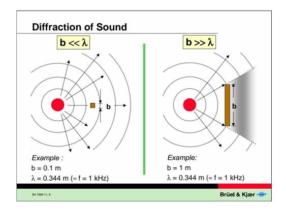
Objects placed in a sound field may cause diffraction.
