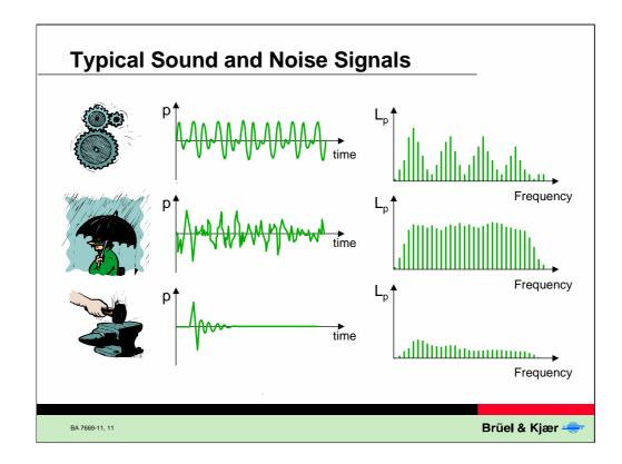
Most natural sound signals are complex in shape. The primary result of a frequency analysis is to show that the signal is composed of a number of discrete frequencies at individual levels present simultaneously.
