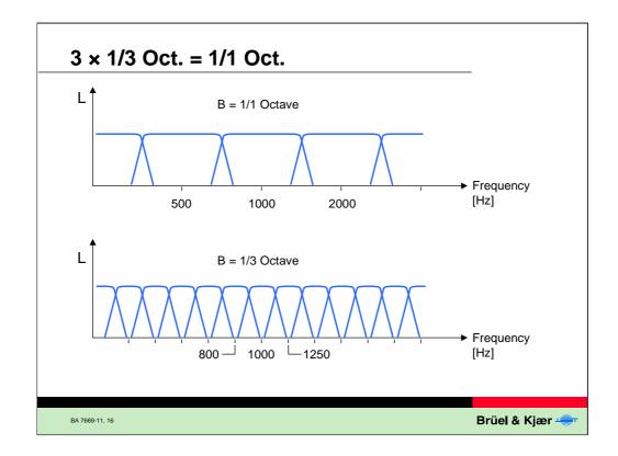
One advantage of constant percentage bandwidth filters are that e.g. two neighbouring filters combine to one filter with flat top, but with double the width. Three 1/3 octave filters combine to equal one 1/1 octave filter.
