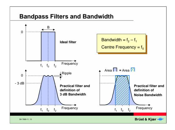
Ideal filters are only a mathematical abstraction. In real life, filters do not have a flat top and and vertical sides. The departure from the idealised flat top is described as an amount of ripple. The bandwidth of the filter is described as the difference between the frequencies where the level has dropped 3 dB in level corresponding to 0.707 in absolute measures.
