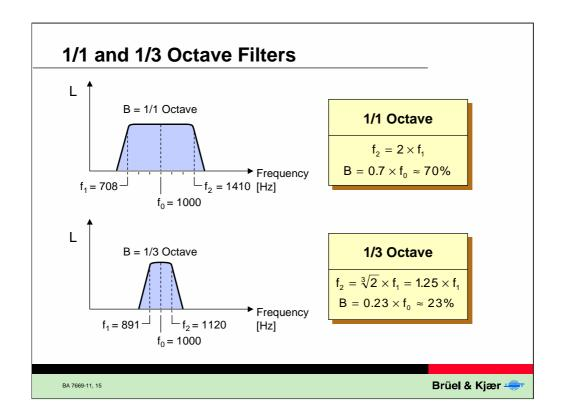
The widest octave filter used has a bandwidth of 1 octave. However, many subdivisions into smaller bandwidths are often used.
