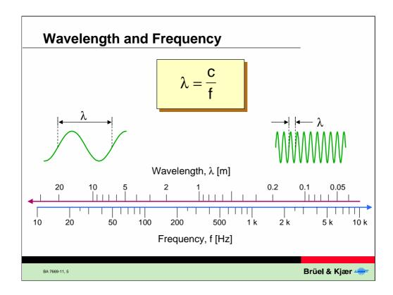
The wavelength, the speed of sound and the frequency are related according to the formula shown.
