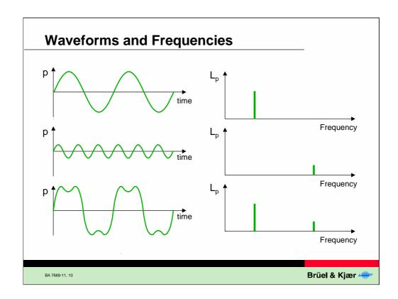
Three examples of the relationship between the waveform of a signal in the time domain compared to its spectrum in the frequency domain.
