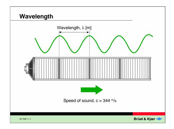
A sound signal from a loudspeaker mounted at one end of a tube will produce a sound wave that propagates forward at a speed of 344 m/s.
