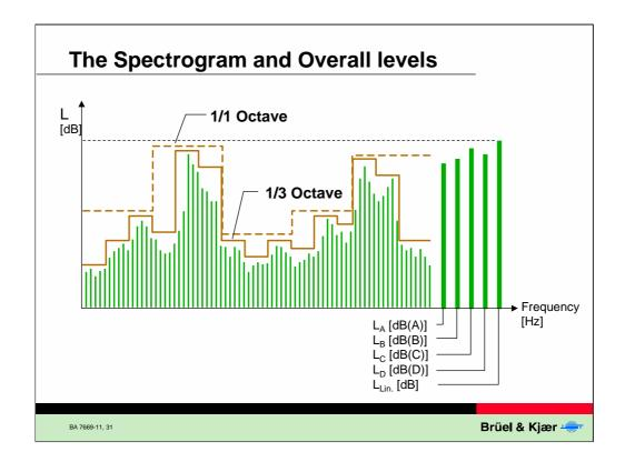
The advanced sound level meters often feature comprehensive displays showing all the analysis results from both the parallel analysis filters and the weighting curves simultaneously.
