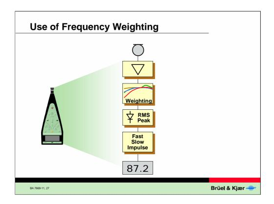
All sound level meters have built in A-weighting, and some have also others like B and C-weighting.
