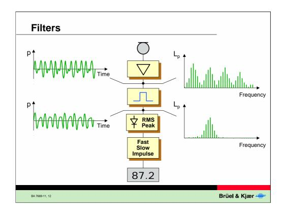
To analyze a sound signal, frequency filters or a bank of filters are used. If the bandwidths of these filters are small a highly accuracy analysis is achieved.
