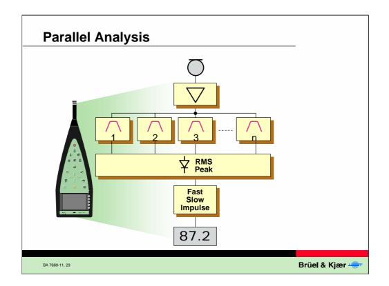
A sound level meter with a parallel filter bank is the most expensive, but the fastest in operation and does not require the signal to be stationary.
