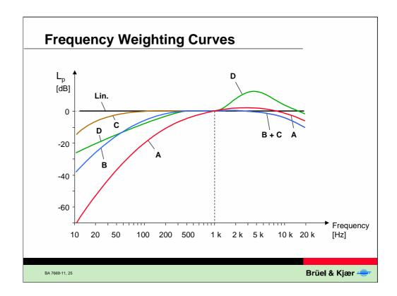
The A-weighting, B-weighting and C-weighting curves follow approximately the 40, 70 and 100 dB equal loudness curves respectively.
