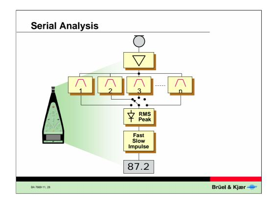
For more detailed frequency analysis sound level meters can have a serial filter bank of 1/1 octave and maybe also 1/3 octave bandwidths. As only one filter is active at a time the analysis time is long and requires the sound field to be stationary. The advantage is a lower price.
