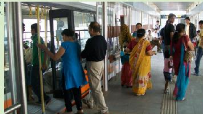
Platform-level boarding speeds boarding and alighting in Ahmedabad, India.
