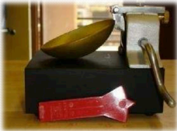
Casagrande Equipment to determine Liquid Limit
