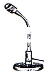
Unidirectional dynamic microphone
