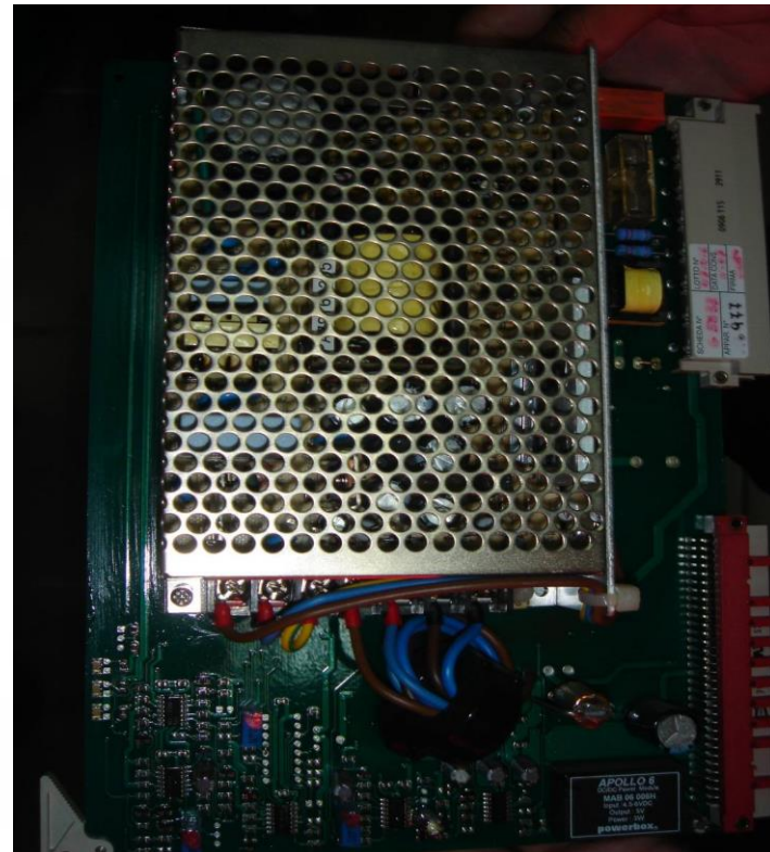
Power Supply Card Unit
