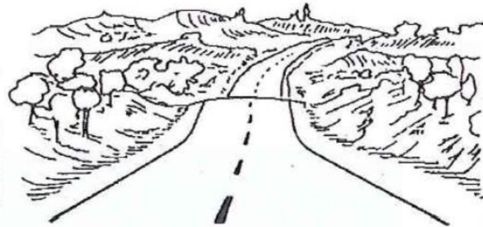
Figure 7: Both examples have visually poor alignment with unrelated horizontal and vertical curves and broken backed horizontal curves
