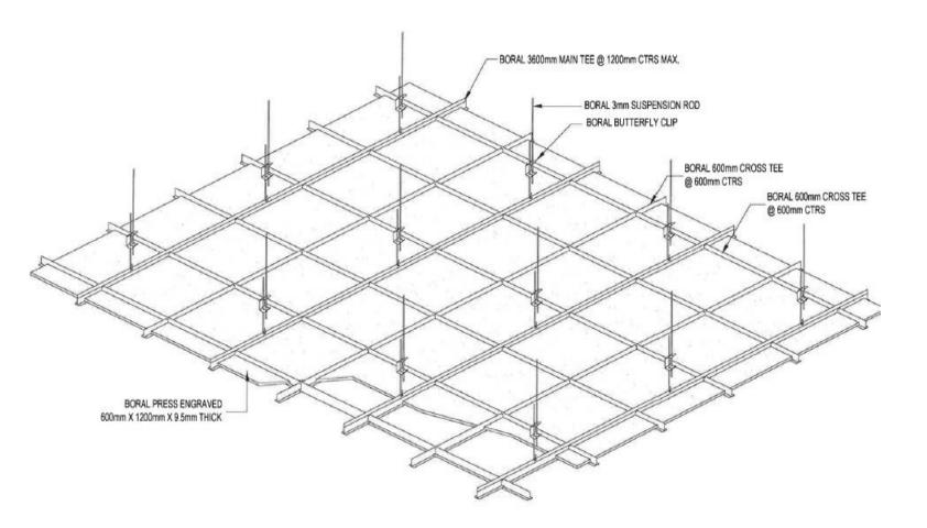
Suspended Exposed Grid Ceiling 600mm X 600mm X 9.5mm thk Press Engraved Gypsum Board with Anti-Fungus Paint (GB1)
